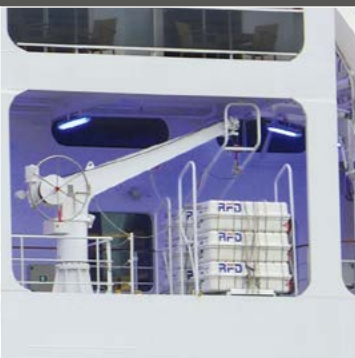
Davit using slew drive
